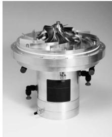
The turbo-blower for cooling a laser ( $CO_2$ ). Speed is 54000 rpm , the rotor mass is 3.6 kg, the motor power is 12 kW, the radial bearing diameter is 48 mm, the bearing force is 230 N (TRUMPF/MECOS).
