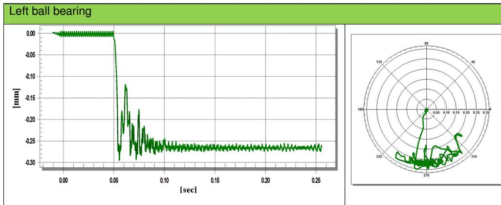
Fig. 13 The rotor drop on the rolling bearings
