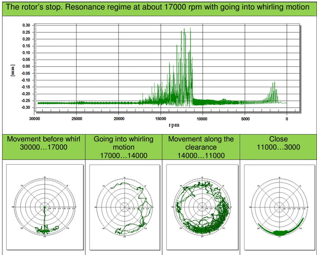
Fig.15 The rotor's runout and whirl effect
