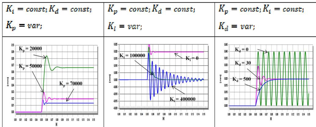
Fig.3 Impact of the control factors on the dynamic system when the static force appears
