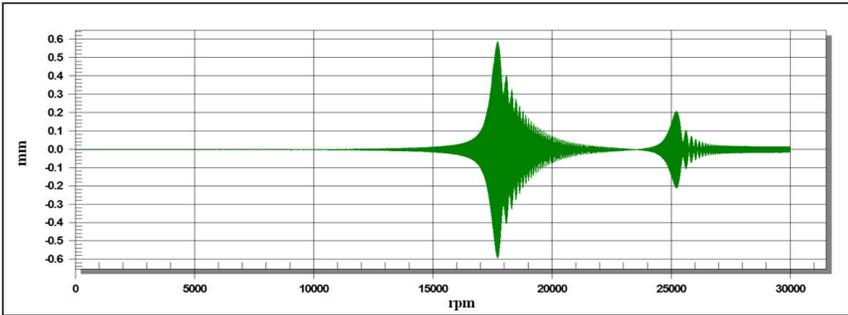
Fig. 8 Amplitude-frequency response at unsteady analysis, left AMB section
