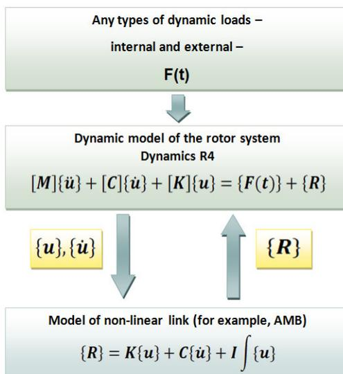
Fig.4 Scheme of interaction between the rotor system's dynamic model and non-linear elements
