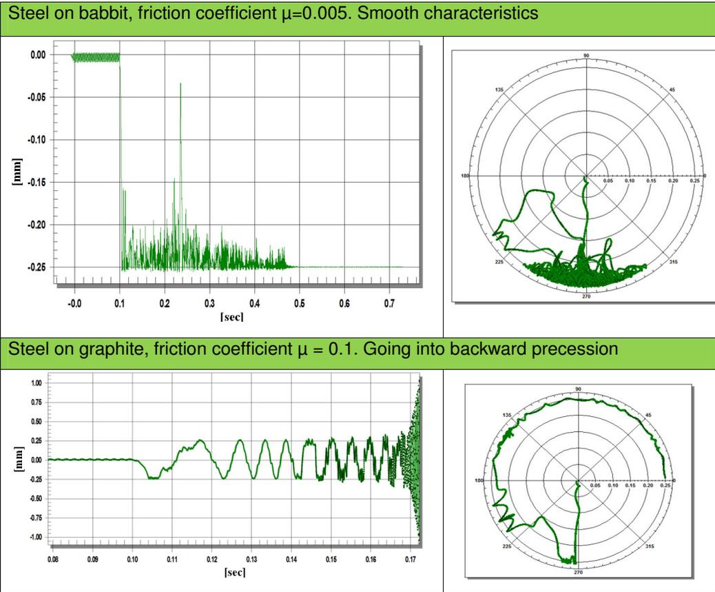
Fig. 12 The rotor drop on the journal bearing. Left bearing
