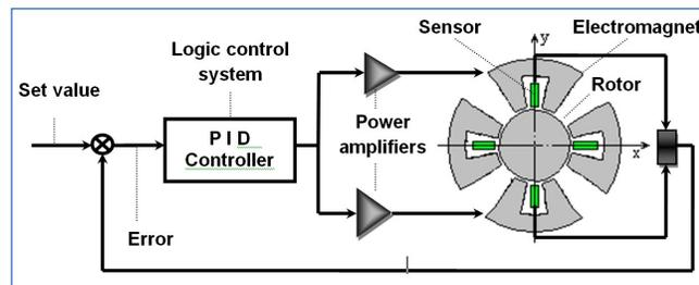
Fig. 2 Scheme of AMB operation
