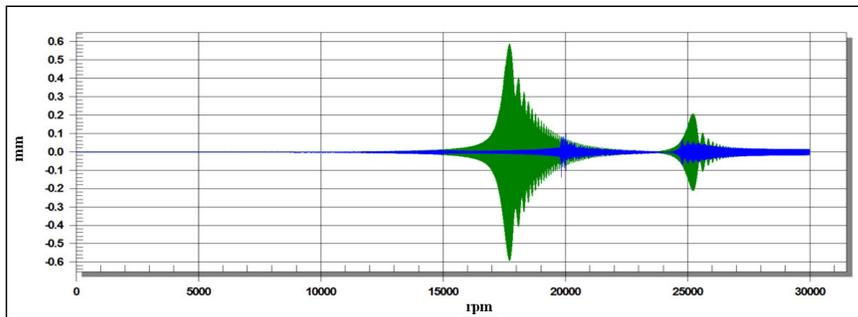
Fig. 11 Results of going into the regime with the chosen program of the stiffness control
