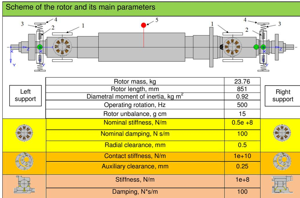
Fig. 6 Scheme of the rotor and its main parameters
