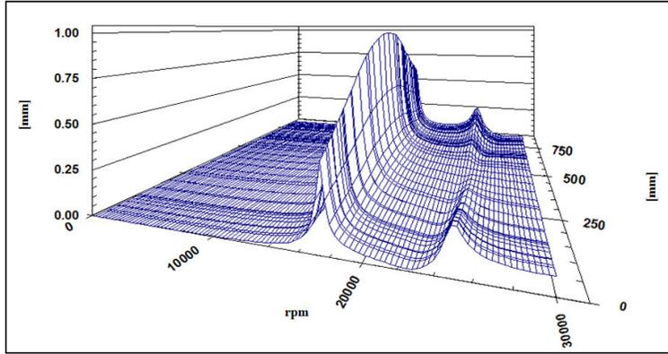
Fig.7 The rotor's amplitude-frequency response
