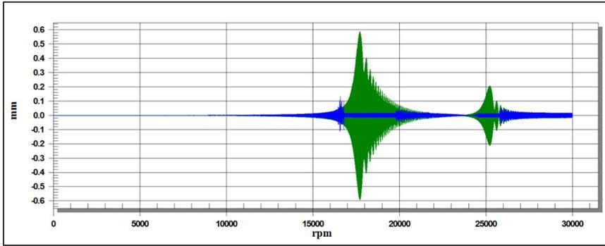
Fig. 9 Results of achieving the regime with the chosen program of damping control
