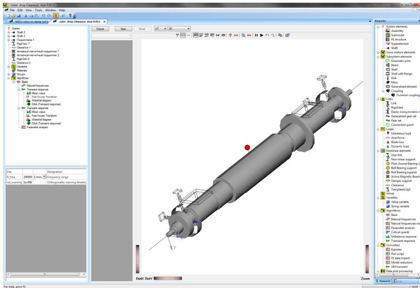
Fig. 4 The main window of the Dynamics R4 software with the investigated rotor supported by AMB
