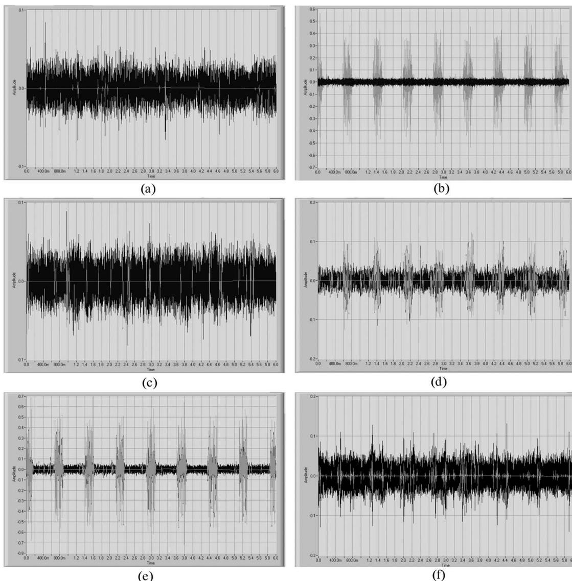
**Fig. 8. Results of processing of a signal obtained during the testing of a variously damaged bearing:**
