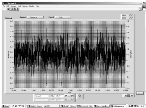
**Fig. 3. Oscillogram of a good state bearing. Regime 1**
