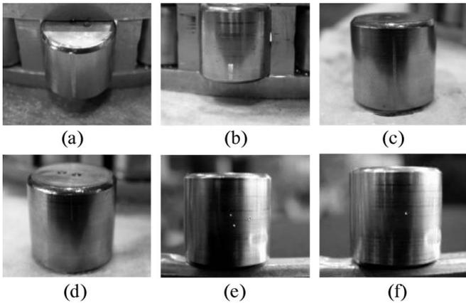
**Fig. 2. Damages of rollers according to the measurement data.**
