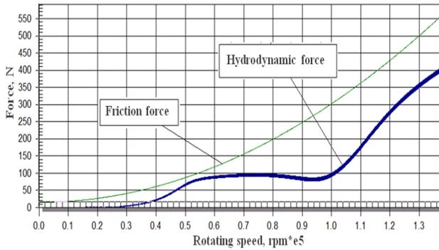
Figure 16 Forces acting on seal ring S5
