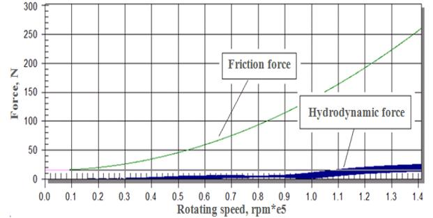
Figure 12 Forces acting on seal ring S5
