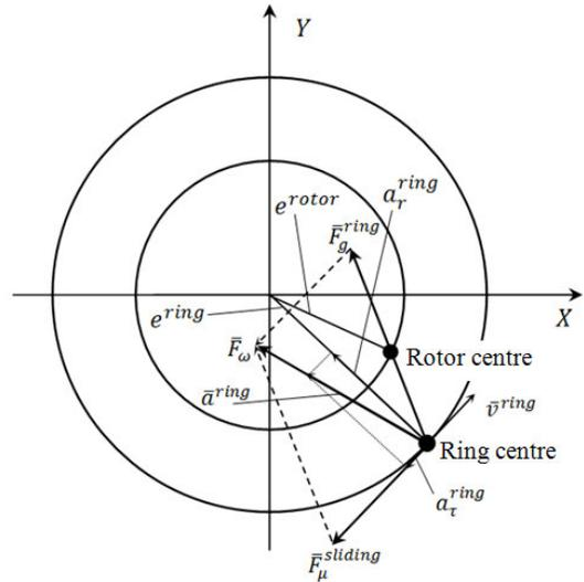
Figure 10. Vector scheme of ring motion
