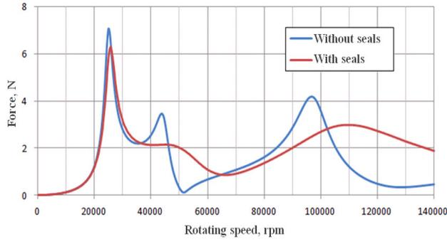
Figure 5. Loads in section elastic-damping support 1
