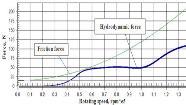
Figure 17 Forces acting on seal ring S6
