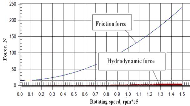
Figure 15 Forces acting on seal ring S4
