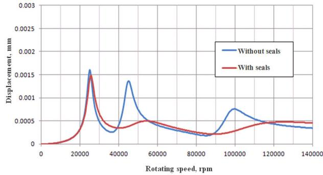
Figure 7. Displacement in section 1 of turbine stage
