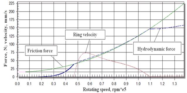
Figure 19 Forces acting on seal ring S8
