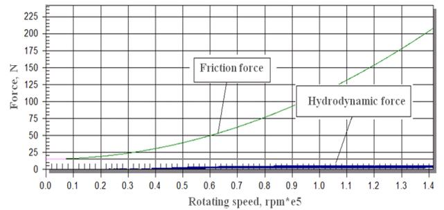
Figure 13 Forces acting on seal ring S8
