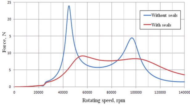
Figure 6. Loads in section elastic-damping support 2
