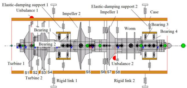
Figure 2. Model of turbopump rotor
