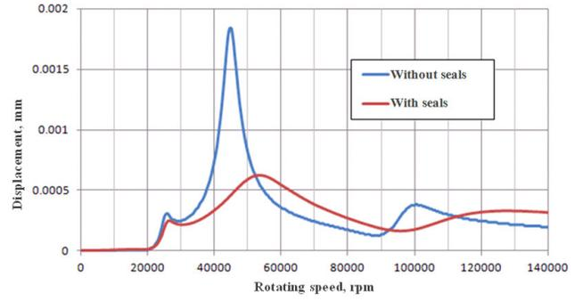
Figure 8. Displacement in section 1 of pump stage
